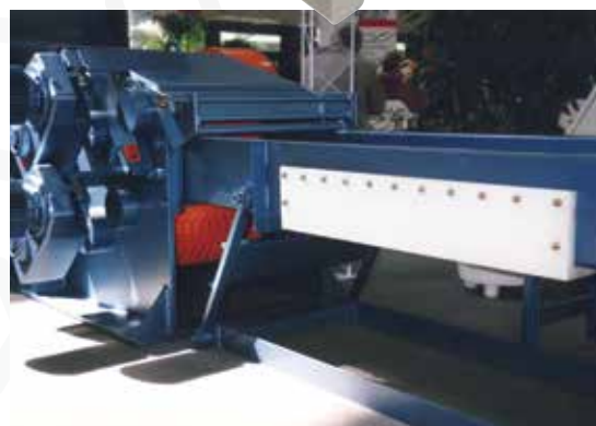
Model VC Eriez Metalarm installed on a vibrator conveyor protecting a chipper
